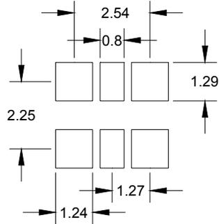
Note: LVDS VCXOs are designed to fit on Industry standard, 6 pad, layouts.
